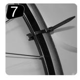
Fasten wheels in position using the supplied zip ties
